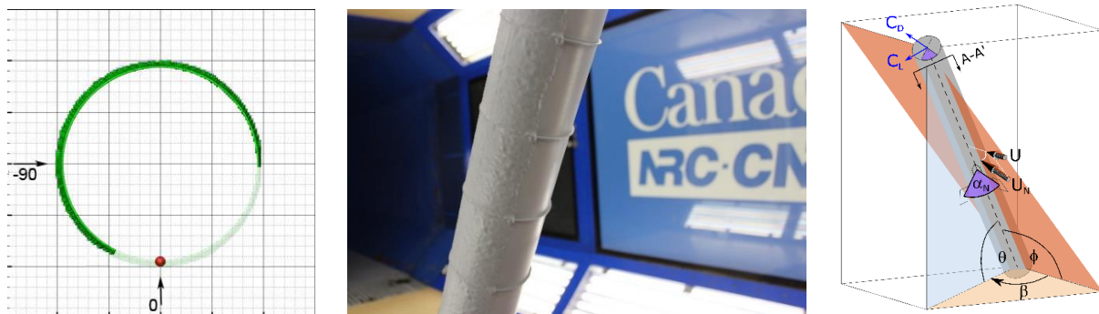
Figure 2. Left: cross-sectional view of the cable with the ice covering the circumference shown in dark green, Middle: Close-up view of one cable model installed in the wind tunnel, Right: Schematic of cable-wind orientation.
