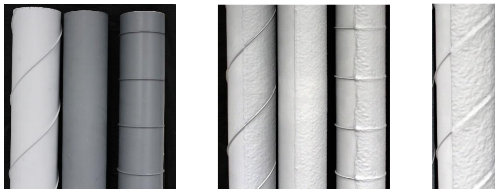
Figure 1. Left: cable models for dry-wind conditions with helical fillet, bare surface and concentric rings. Middle: cable models with thin simulated ice, Right: cable model with thick simulated ice.
